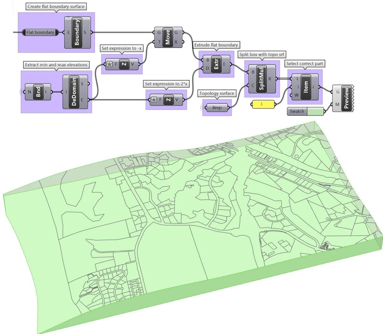
If you acquire the shapefile for the surrounding buildings, then you can also create the .mkgis and add to the model the same way as the parcels and topography, You can then create the 3D geometry of the surrounding buildings by extruding their footprint using the elevation value.
