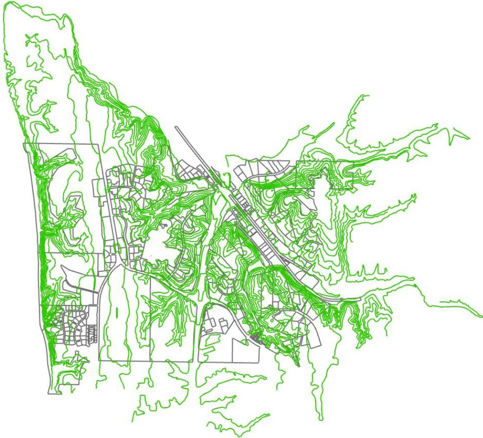
Use the elevation data per contour to place in the proper vertical location, then use **Patch** to create a surface through the contours. You can then project the outline to the patch.
