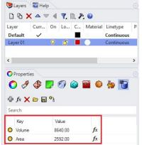
When scale the box, the area and volume recalculates dynamically and display in the user text area
