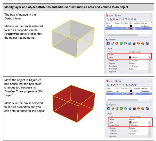
Add user text to calculate the surface area of the box and attach to the object using the User text tab in the **Properties** panel, then:
