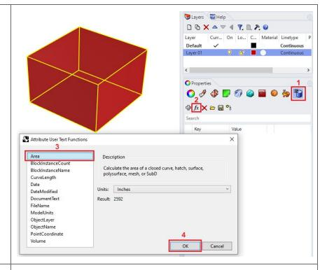
The area and volume are calculated and displayed in the Key/Value box of the user text properties.
